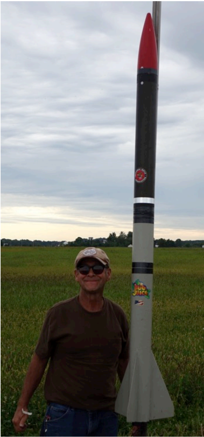
(Above left) Mark Coburn flew his LOC/Precision "Expediter-EXP" on an AT I211 motor to an altitude of 3500 feet.
