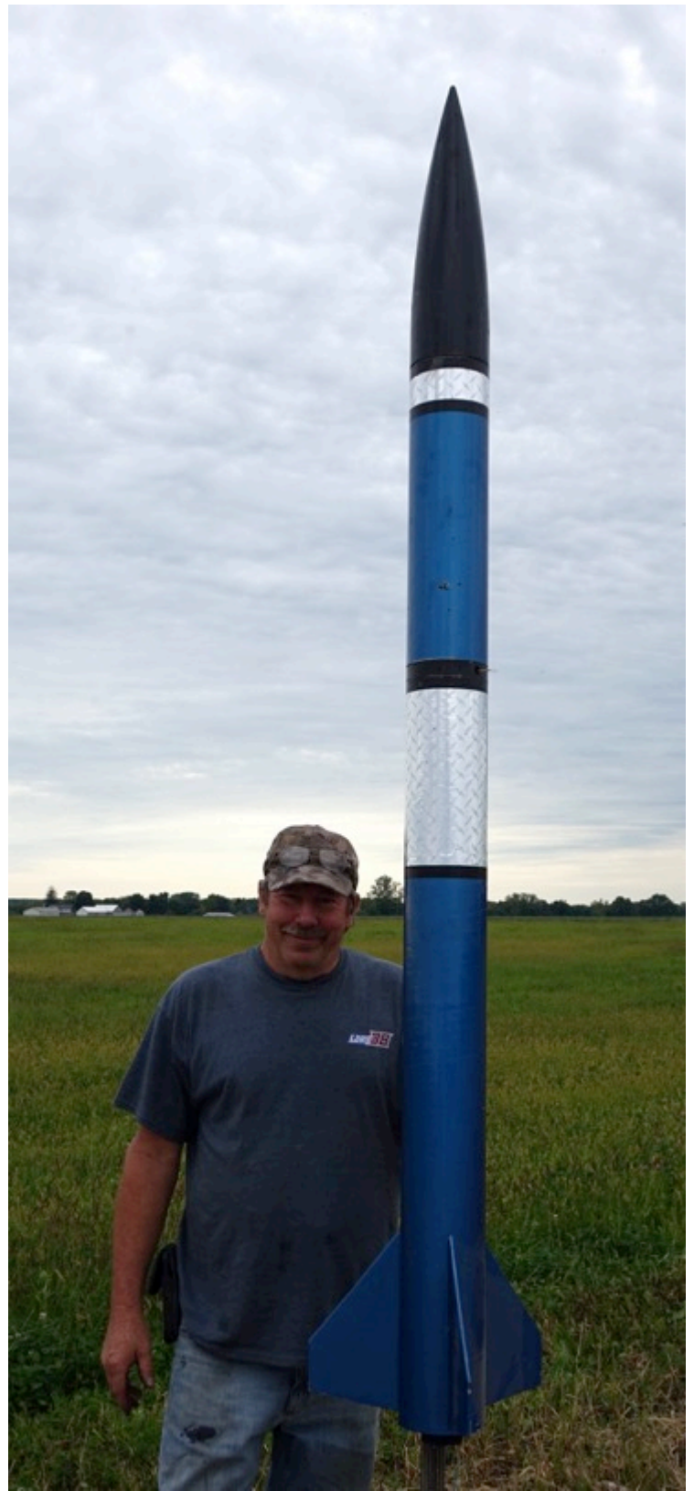
(Above left) Mark Coburn flew his LOC/Precision "Expediter-EXP" on an AT I211 motor to an altitude of 3500 feet.
