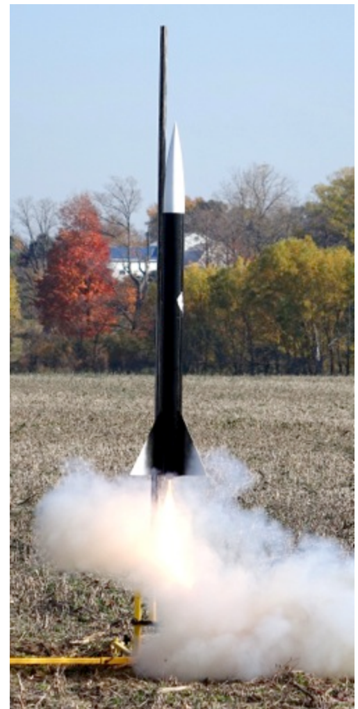
Austin Conn flew his 4" scratch built rocket with AT H135W motors (right). He did three flights with the same rocket, and had one hard landing for lack of proper parachute deployment but the damage was easily repairable.
