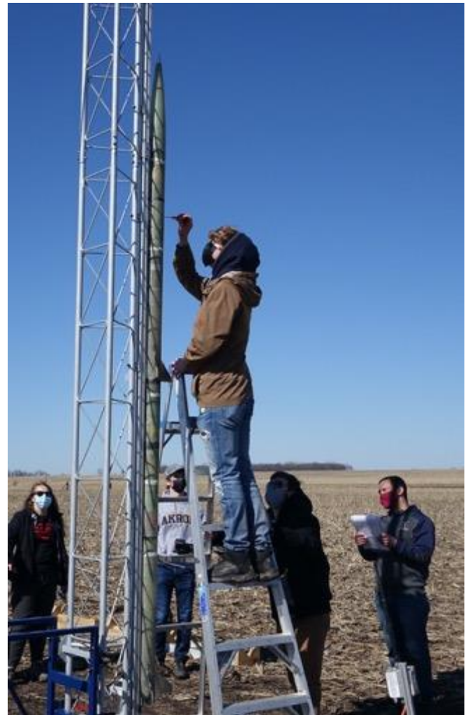
The two-stage rocket was powered by a CTI K1440 motor in the first stage, insuring plenty of power to get to staging altitude and a K250 on the sustainer.
