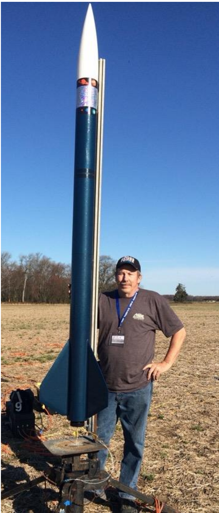
Steve Eves with his LOC/Precision "HyperLOC 1600" which he flew with a 75mm EX L1300 Purple motor to an altitude of 6580 feet.
