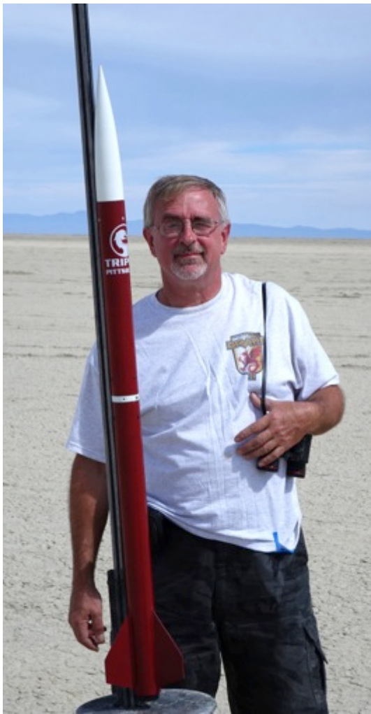
Larry Benek (left) brought out his 4.15 lb. 54mm rocket called "Red White" with a 38mm I348 motor packed with NASSA Slow propellant. His rocket hit an altitude of 6668 feet.
