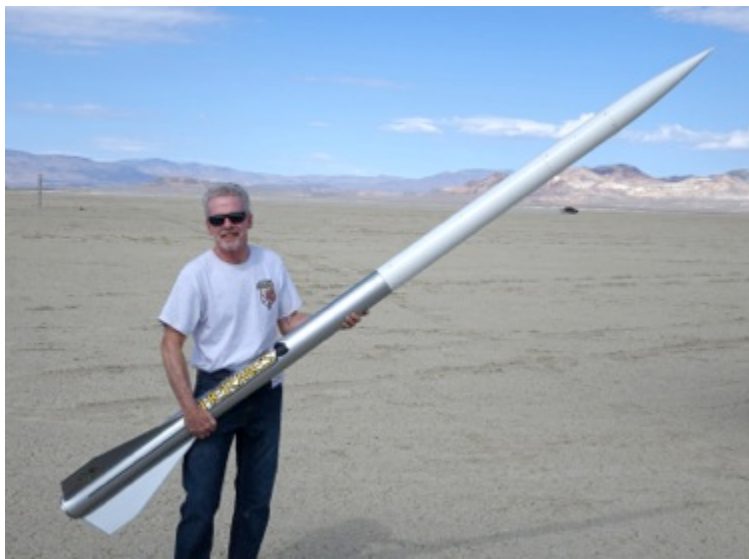
NOTRA member Ken Good (above left) on the way out to the launch pad with his "Hermes" 4" diameter rocket powered by a Research M2107 NASSA Red motor, which flew to 17,863 ft. at Mach 2.1. Chris Pearson (above right) proudly poses with his newly acquired Darque Star "Obsidian" almost all aluminum rocket. Chris will be returning with it next year to fly it with a baby N motor. Fully loaded with propellant it would come out to be an "O" motor.
