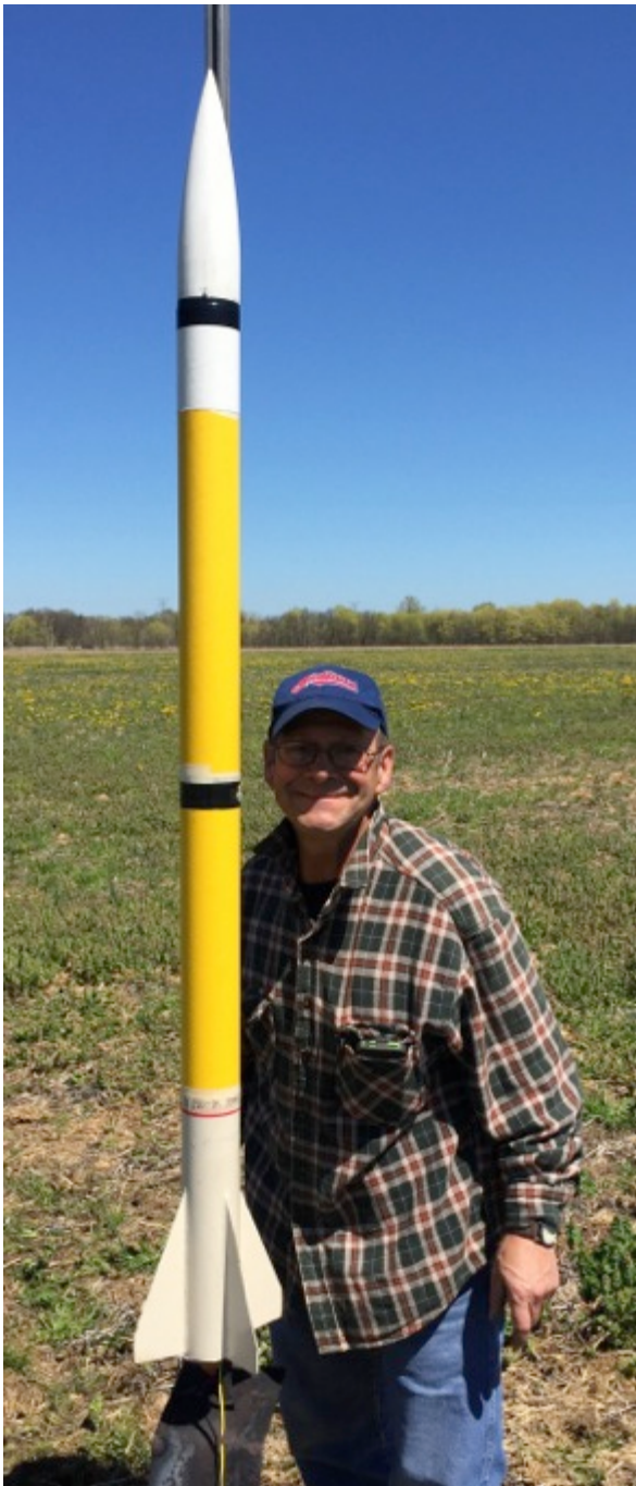
Mark Coburn with his LOC/Precision "Forte" (above) which he flew with an AT H128, which hit 1800 feet and was recovered by dual deployment near the pads.
