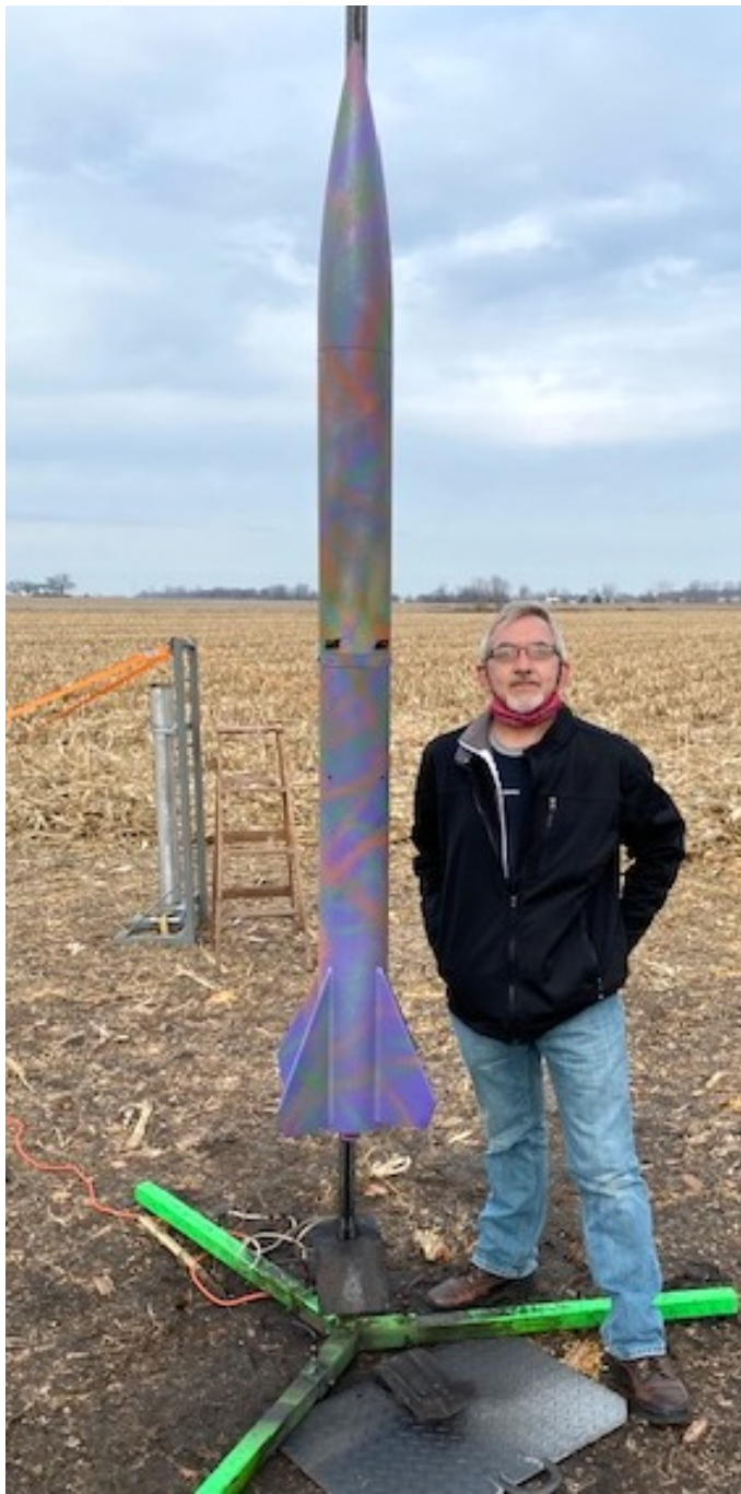
Jim Siebyl (left) with his scratch built rocket "Purple Haze", which he flew on an AT L1000 motor going to an altitude of 6834 feet.
