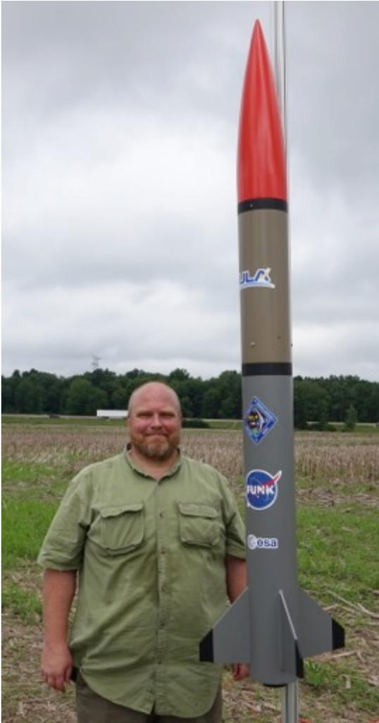
Andrew Kleinhenz (left) flew his 5.5" diameter, 6 foot tall rocket called "Earth, Wind and Fire" hence the "Funk" sticker on it. It flew on a Research 54mm three grain RCS Purple for a perfect flight to 2970 feet. Then another flight on a 54mm 3 grain NASSA K2 Fast which weathercocked badly and nearly landed on the turnpike.
